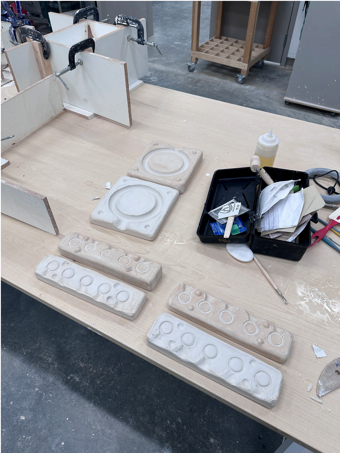
Fig. 16. Claudia Goulet-Blais, Process Image (mold making for slip casting porcelain) , 2024.
