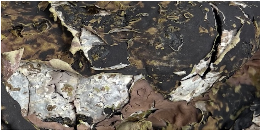
Figure A.4d. Post-Firing Surface of Modified Clay Body
